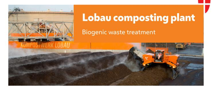
The Lobau composting plant turns biogenic waste collected in the bio-waste bins in the green belt and less densely populated parts of Vienna, at waste treatment centres, and by the Vienna Parks and Gardens (Municipal Department 42) into compost by means of open composting. The compost is used in organic farming and to produce garden soil, and is available for free at many Vienna waste collection centres.
