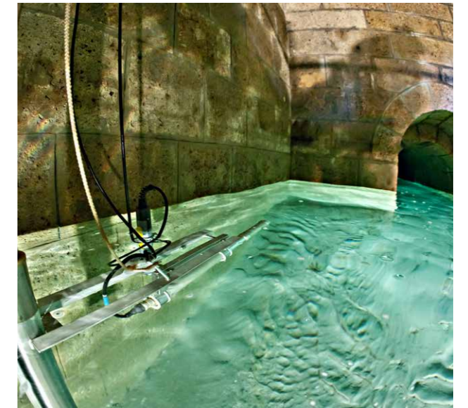
Measuring device for real-time water quality monitoring directly in the spring
