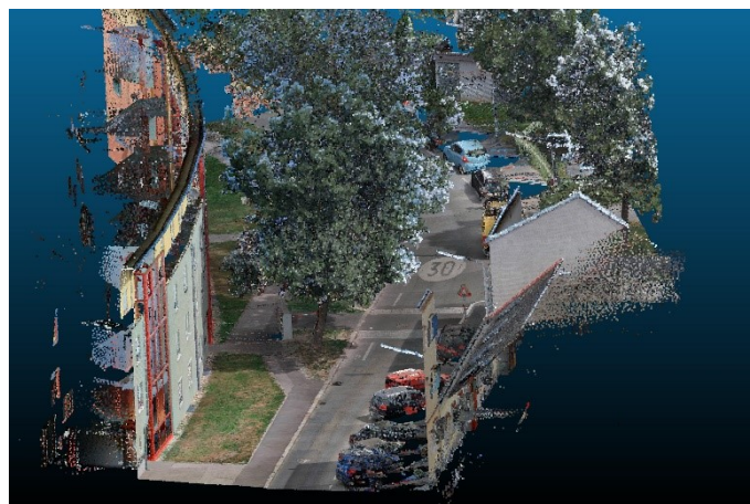
Bottom: Rendering of a section of the LIDAR point cloud
