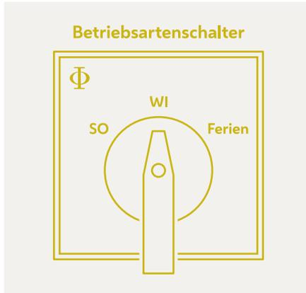
A simple switch: This switch allows even laypeople to operate the HVAC system safely and easily, switching between winter, summer and holiday mode. This saves energy and costs. The primary school in Krottenbachstraße in the 19<sup>th</sup> district, for example, was equipped with this switch, ensuring energy-efficient operation.
